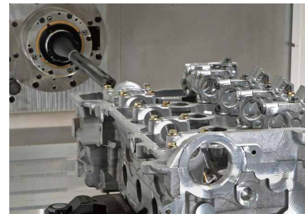
Fine line boring for camshaft bearing bores
